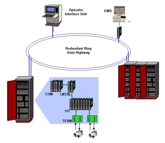
Figure 1: Example First Generation DCS
