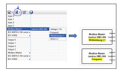
The incoming signal (from the Janitza PQ Analyzer) can be communicated through an IEC 60870-5-104 server or an IEC 61850 server as depicted below. The same signal may be communicated for different use-cases simultaneously.
