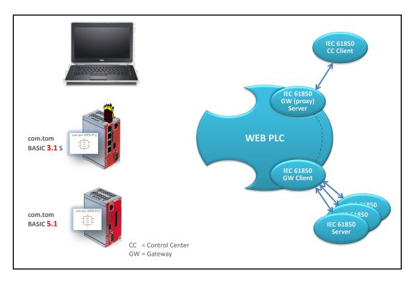
The example in the following figure models and creates an IEC 61850 proxy server that "mirrors" the underlying fan heater status (fan heater operational status). The com.tom BASIC 3.1 S acts as an IEC 61850 client to two IEC 61850 IEDs: com.tom BASIC 5.1 with the IED name "PQServ" and DK61 with IED name "DK61". These two IEDs implement each an IEC 61850 server.
