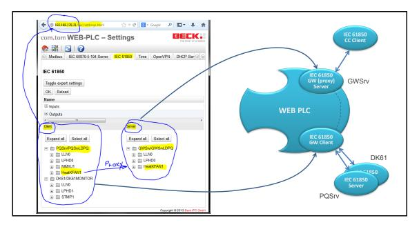
The internal "link" between the fan heater status coming from the underlying IED and the server for the uplink is configured by drawing a line between the input signal and the output
