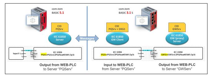
The heater fan status object at the WEB-PLC is an output object as shown on the left side (in the com.tom BASIC 5.1) and representing an IEC 61850 status object of the server "PQServ". This status is reported by a message to an IEC 61850 client in com.tom BASIC 3.1 S and exposed as an input object at the WEB-PLC. This input object is finally marshalled to an output object (to the IEC 61850 proxy server "GWSrv") in order to report the value to a higher level IEC 61850 client (not shown here).
