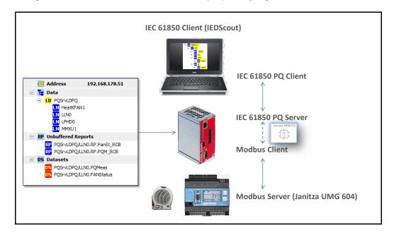
The signals for the most known measurements in the power systems are standardized in IEC 61850 as logical nodes (e.g., MMXU) that contain data objects (e.g., TotW and Hz). Most of
