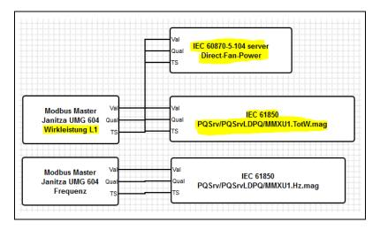
The signal list for the IEC 60870-5-104 server has also to be configured manually by filing out a form at the web browser. The WEB-PLC object "Direct-Fan-Power" (configured for the WEB-PLC) is communicated as a measurement value with IEC 60870-5-104 message type identifier 34 and information object address 5102:
