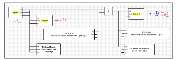
Any other reasonable application can be configured graphically by placing signals on the work space and connecting them with functions (e.g, an OR gate) and other signals.
