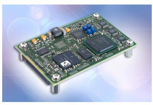
Hirschmann<sup>TM</sup> has added the new managed Embedded Ethernet switches EES 20 and EES 25. (Photo: Belden, PR213)
