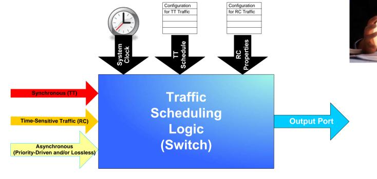
Ethernet switch can predict future collisions, plan for their resolution, and protect time-critical and time-sensitive traffic!
