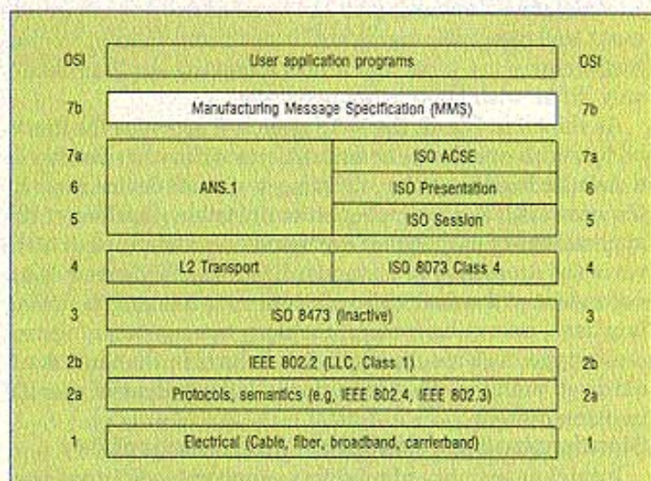
Fig. 1: The MMS specification defines machine-specific functions and applications for the manufacturing world. The International Standards Organization in its OSI model has begun standardizing communications among plant floor devices.
